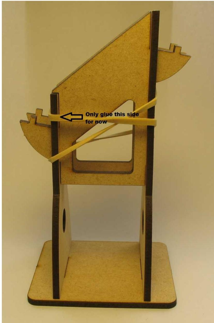
Insert the camshaft between the frames so the crank handle cut-out is on the tall upright side. Glue the tall upright to the side frames and glue the upright to the base. Leave to dry.
