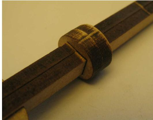
Slide on a cam, two spacers and another cam, ensuring the cam is 180 degrees rotated in relation to the first cam. Repeat until all cams and spacers have been used.
