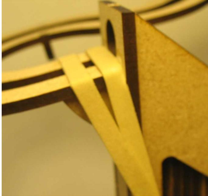
Once the top end of the track is securely mounted you can attach the lower part to the frame. If using a slow drying/setting glue it should be held firmly in place while the glue sets. Use a scrap of MDF and strong rubber bands. Take care not to glue the scrap piece onto the track.
